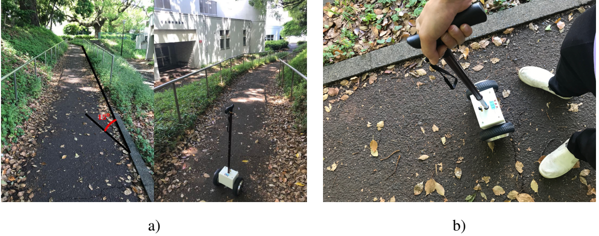
Figure 5.7: Two-wheeled cane in self-balancing mode (a) and help the user to walk on slope environment (b).
