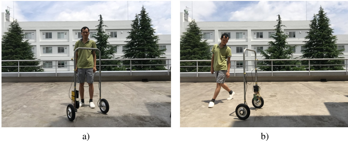
Figure 5.9: Self-balancing mode of the two-wheeled walker: (a) at the 1 st second; (b) at the 45 th second.
