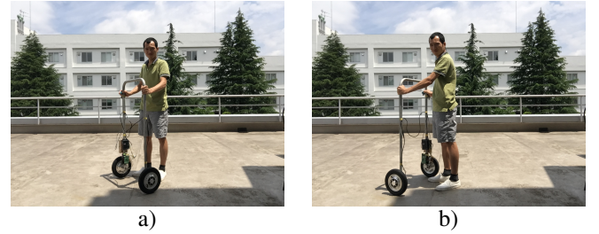
Fig. 6. The status of the two-wheeled walker when the user walk: (a) move forward; (b) move backward.
