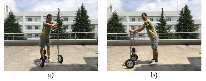
Fig. 5. The status of the two-wheeled walker when the body weight is put on it: (a) the whole body; (b) a half of the body.
