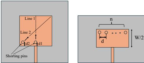
Fig. 3. Cases adding shorting pins: (a) one pin on Line 1 and Line 2 (b) an array of  $n$  shorting pins.
