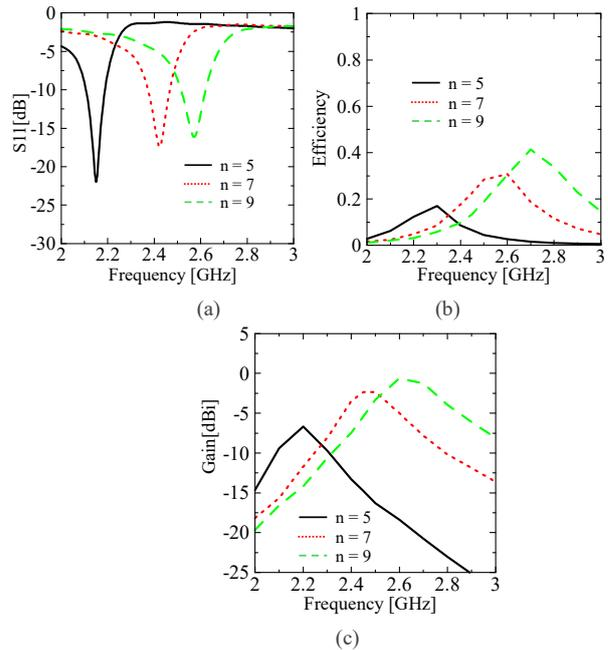
Fig. 5. Simulation results in S11, efficiency, and gain of the antenna with an array of  $n$  shorting pins.
