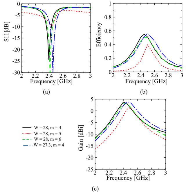
Fig. 10. Simulation results in S11, efficiency, and gain when  $m = 4, 5, 6$ .
