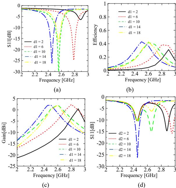
Fig. 4. Simulation results in S11, efficiency, and gain of the antenna adding a shorting pin on Line 1 and Line 2.
