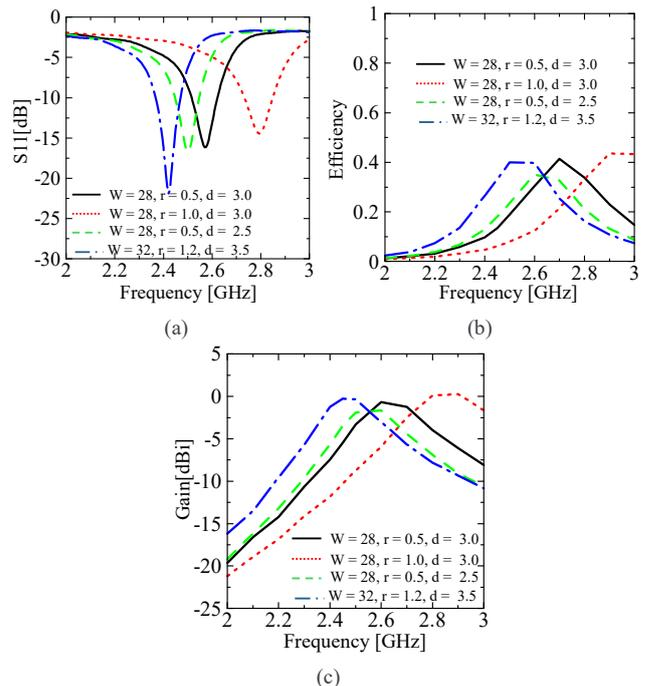
Fig. 6. Simulation results in S11, efficiency, and gain when  $d$  and  $r$  changes.
