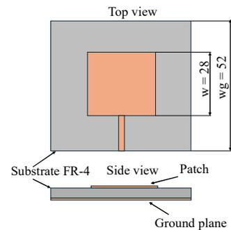
Fig. 1. A square microstrip antenna at 2.45 GHz using FR-4 substrate.
