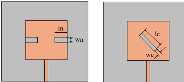
Fig. 7. Configurations of slots on the patch: (a) two notches ( $W = 23.7$ ,  $w_n = 5.85$ ,  $l_n = 2$ ) (b) one slot on the diagonal ( $W = 28$ ,  $l_c = 10$ ,  $w_c = 1$ ) (unit: mm).
