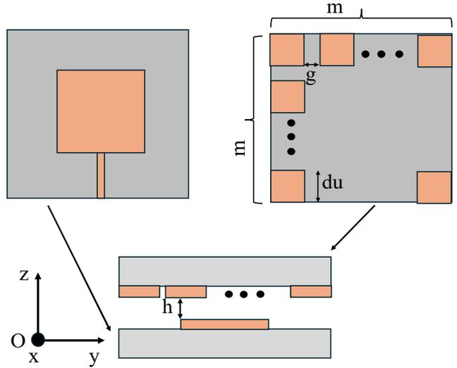
Fig. 9. Structure of the antenna with a simple metasurface.
