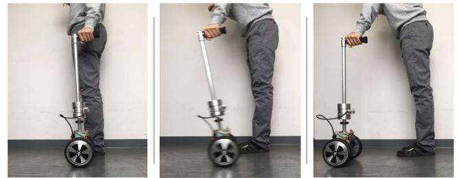
Fig. 14. The two-wheeled cane helping a users balance when they are starting to fall forwards.
