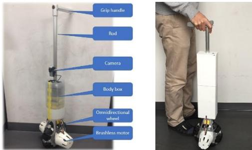
Figure 1: Hardware design of the robotic cane.
