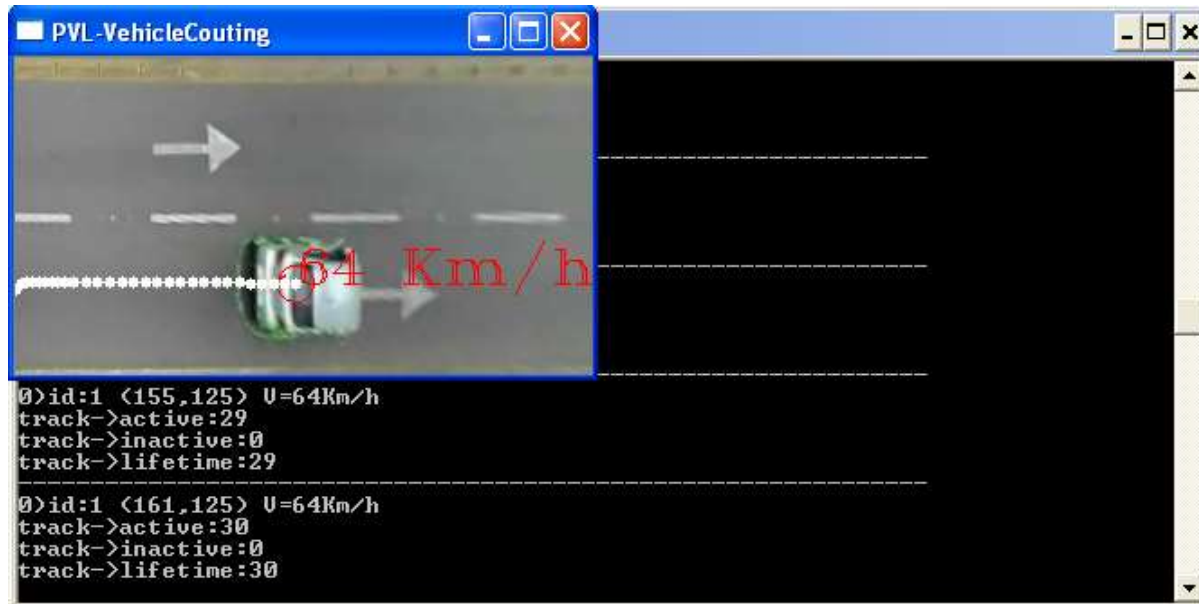
Figure 5. Result of Algorithm tracking speed of the vehicle in each frame.
